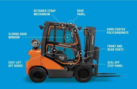
TILTING ROOF PANEL FOR IMPROVED VENTILATION
