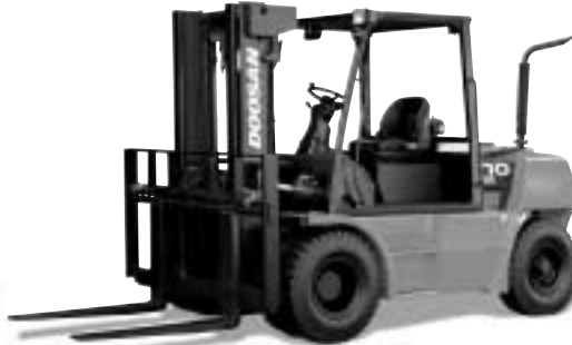
D50S / D60S / D70S-5 & D80S / D90S-5 5,000kg 6,000kg 7,000kg 8,000kg 9,000kg Pneumatic Tire
