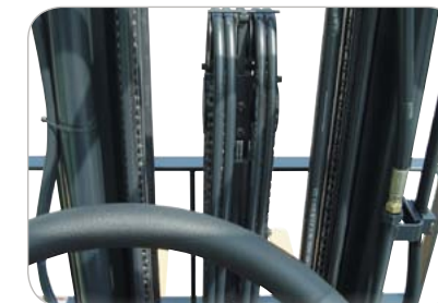
Neatly arranged Hydraulic Hoses Reduce width providing better visibility, silent staging, and added strength.
