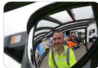
Panoramic Mirror Provides the operator a clear view of the whole back & rear working area, improving, working safety & efficiency.
