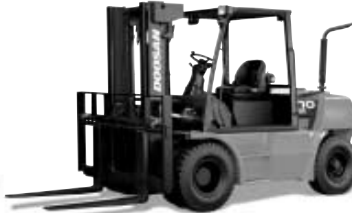
D50S / D60S / D70S-5 5,000kg 6,000kg 7,000kg Pneumatic Tire
